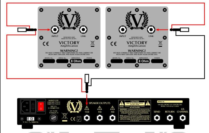
So the end of this lead needs to be plugged into the 16 Ohm speaker socket on the V30. Alternatively, there are speaker matching boxes available. A low cost but reliable example is the Palmer Cabinet Merger, available from many retailers:
