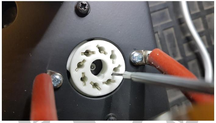
Please make sure you don't close these pins up fully or it will be difficult to replace the Valves. Replacement valves and tools for biasing such as a Multimeter and Terminal Screwdrivers are available directly from Victory. Please email your requirements to <u>service@victoryamps.co.uk</u> for a quote.
